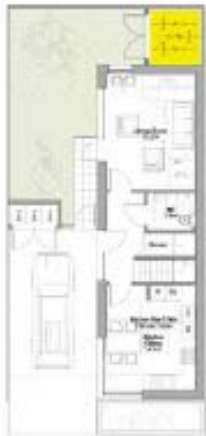
Example of bike storage in a garden shed at the rear of a property
