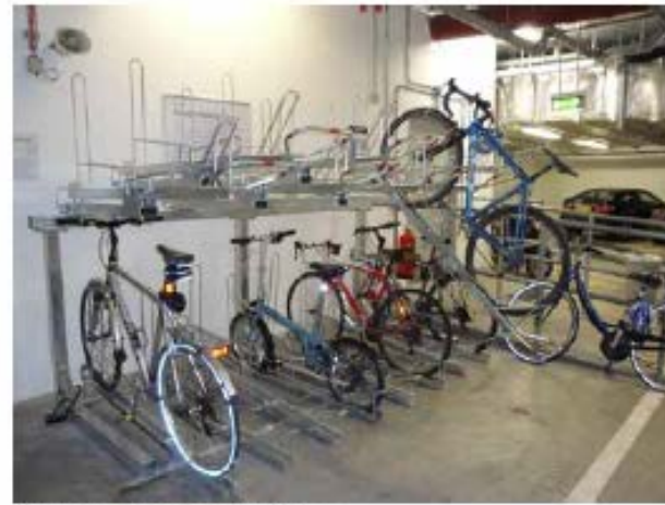
Stacked bike system for apartment buildings
