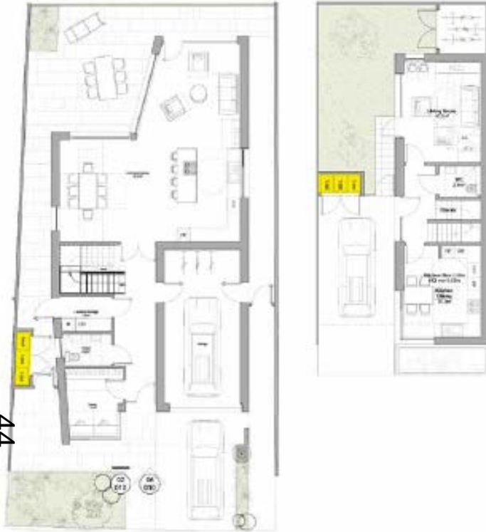
Example of a bin store solution for an individual home. Concealed from the street but conveniently located for residents and refuse collector
